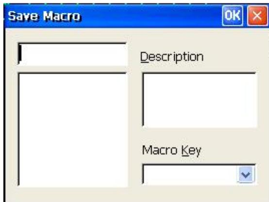
Enter the file name you want the macro saved as. Type the description of the macro for future reference. Assign the macro to a function key (f1-f12) - required if keyboard used to Play back the macro (e.g. ALT+F5 then Fn).
